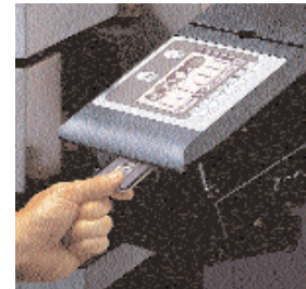
The ability to transfer the PCMCIA card from the programming source to satellite GAGE 2000s adds system flexibility.
